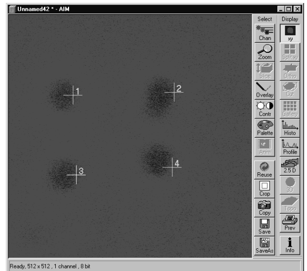
Fig. 5-398 LSM image of the Rh6G layer after bleaching. Deviations between the markers and the bleached spots are noticeable.
